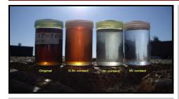
The above Pictures shows the bad oil and the regenerated oil which is as good as new oil. New oil conforms to the standard IEC60296.
